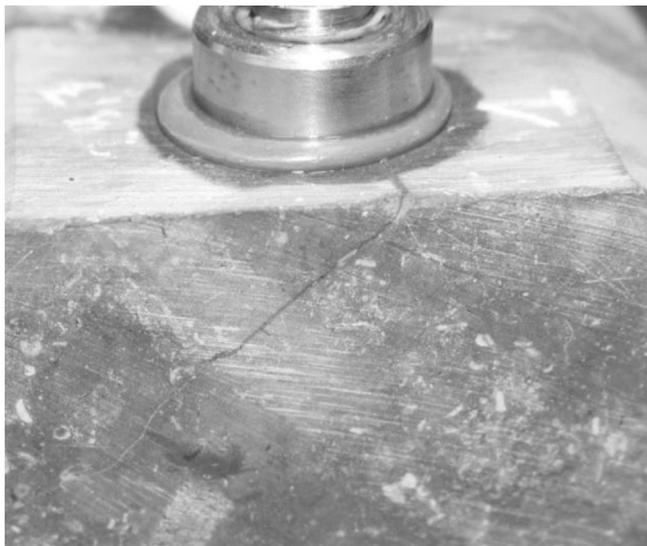
**Fig. 12.** Close up view of the location 1 on the Cobourg limestone; the crack formed near the mini-port connector was accentuated by wetting the surface with water.
