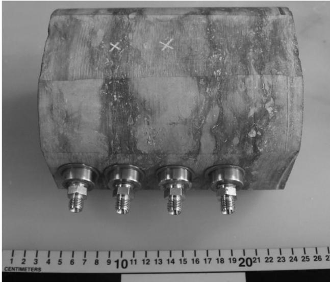
Fig. 1. Cobourg limestone heterogeneous matrix composed of light gray carbonate species and dark gray argillaceous species with installed four mini-port connectors.
