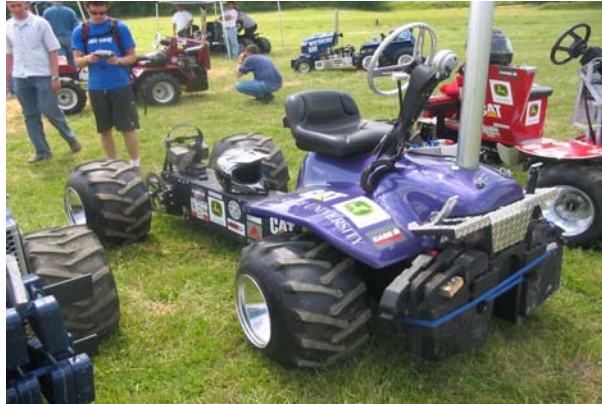
Figure 4. Example of bent sheet metal frame used by Kansas State University.
