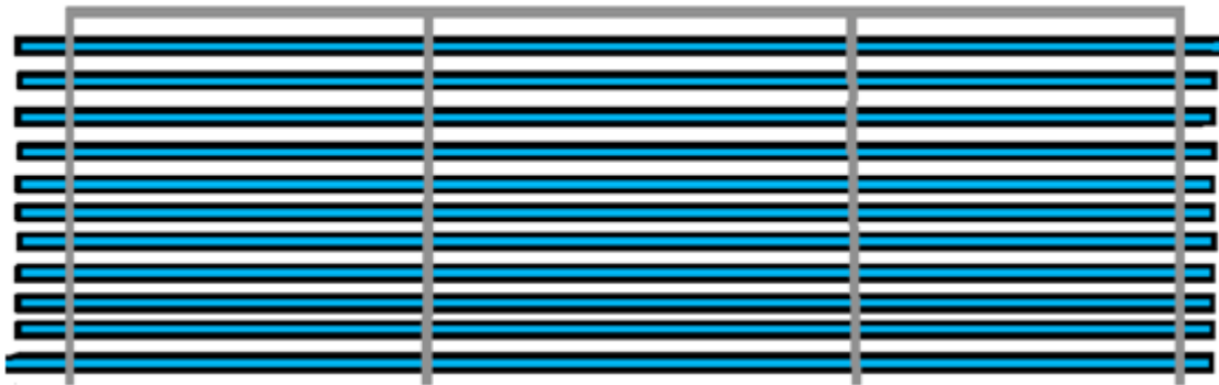
Figure 8. 2-dimensional overview of the flocculation tube system, showing the pipes from the side, with the wastewater entering from the bottom left corner and exiting from the top right corner.
