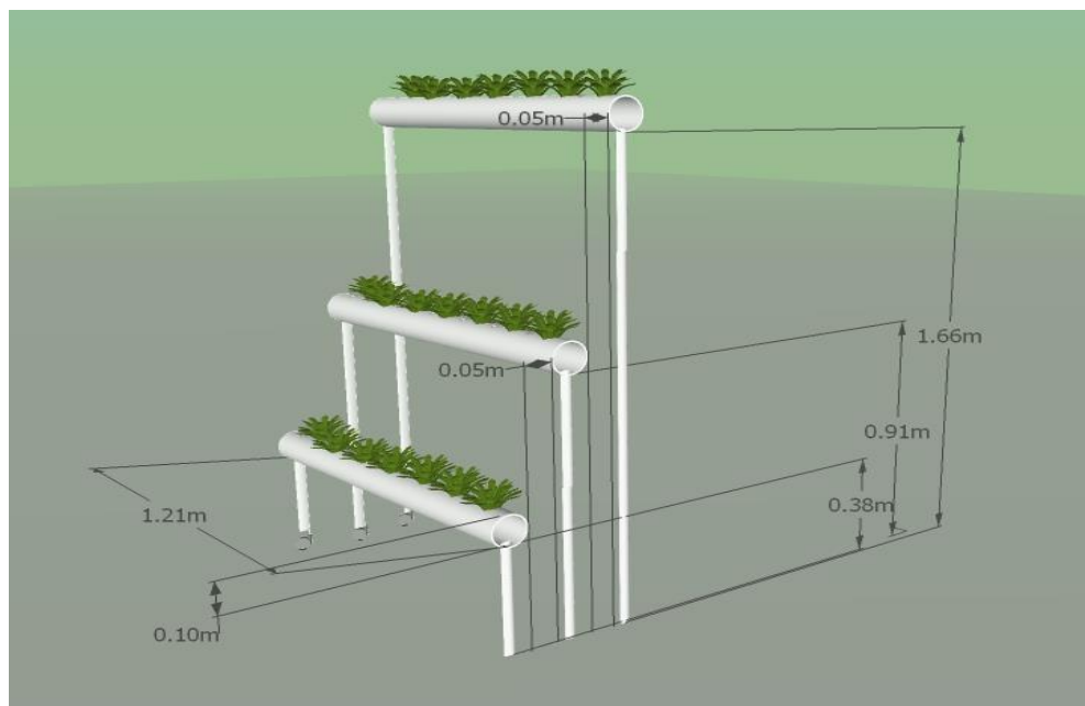
Figure 3. Individual nutrient film technique (NFT) hydroponic pivoting system
