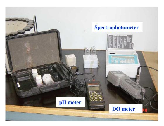
On occasions, an operator needs an indication of water quality "RIGHT NOW". For these situations, sending a sample to the lab, and getting results in a few days, is not an option. (our water treatment plant, or a waste water plant is an example of such a case).
