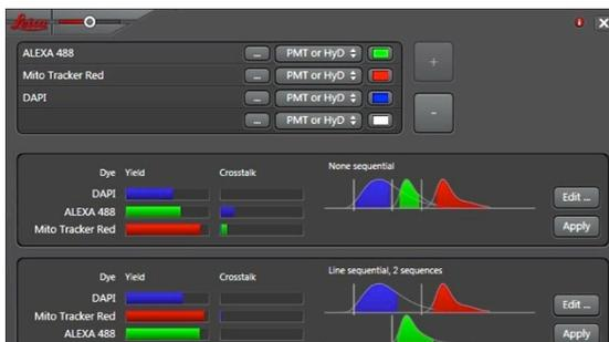
The **Dye Assistant** is a wizard to simplify beam path setup. It is activated using the button labeled '8' above. It allows selecting one or more dyes from the dye database, and a preference of detector. It then suggests settings for acquisition, showing fluorescence yield and crosstalk.
