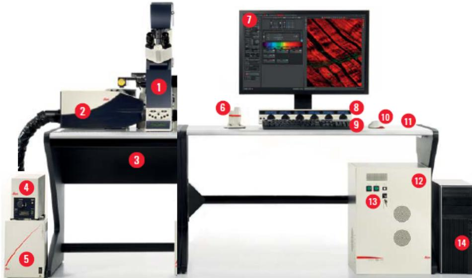
**Fig 1:** Basic components of the Leica SP8 microscope
