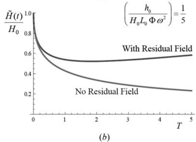
**Figure 6.** Influence of initial hydraulic gradients on the results of conventional 1-D pulse tests. [Initial hydraulic gradient has a sign opposite to the gradient induced by the hydraulic pulse. Result corresponding to equation (28).] (a)  $(h_0/H_0 L_0 \Phi \omega^2) = 1/10$ ; (b)  $(h_0/H_0 L_0 \Phi \omega^2) = 1/5$ , and this 1-D parameter is define by (32).
