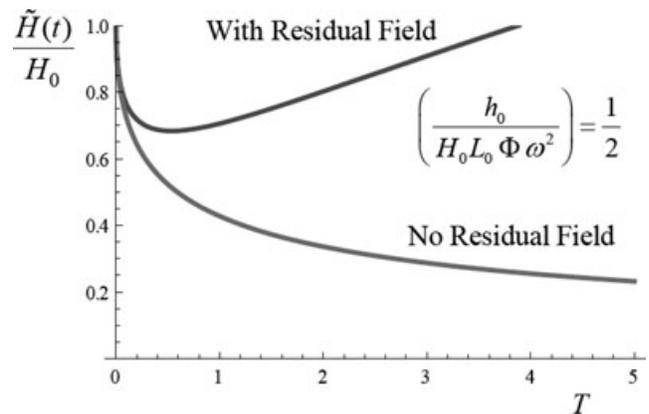
**Figure 7.** Influence of initial hydraulic gradients on the results of conventional 1-D pulse tests. [Initial hydraulic gradient has a sign opposite to the gradient induced by the hydraulic pulse. Result corresponding to equation (28) with  $(h_0/H_0 L_0 \Phi \omega^2) = 1/2$ , and this non-dimensional parameter, is define by (32).]
