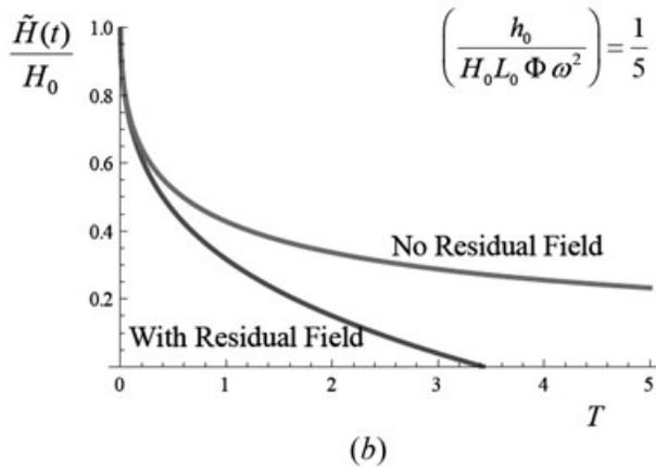
**Figure 5.** Influence of initial hydraulic gradients on the results of conventional 1-D pulse tests. [Initial hydraulic gradient has the same sign as the gradient induced by the hydraulic pulse. Result corresponding to equation (25).] (a)  $(h_0/H_0 L_0 \Phi \omega^2) = 1/10$ ; (b)  $(h_0/H_0 L_0 \Phi \omega^2) = 1/5$ , and this 1-D parameter is define by (32).
