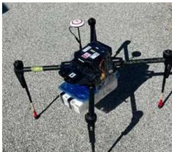
DJI Matrice 100 drone with Multi-GAS sensor attached underneath, used in Campi Flegrei field campaign in March 2004.
