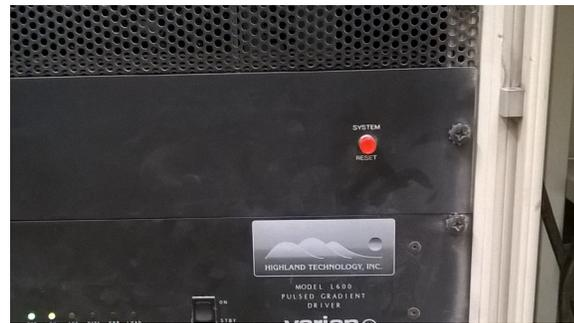
Figure 5: Reset button on Varian Mercury 400.
