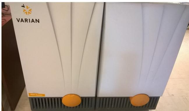
Figure 7: Door of Varian VNMRS console. Open by kicking the yellow panel on the right door.
