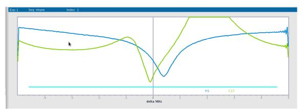
Figure 1. Trtune display for untuned probe. Proton curve is blue, carbon is green.
