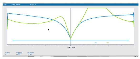
Figure 2. Trtune display for tuned probe: the dips of both curves are in the centre and are deep (nearly touch the bottom).
