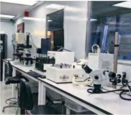
View of several tools: from front to back: stereo microscope, critical point dryer, stylus profilometer, optical microscope, thin film reflectometry.
