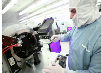
Microfab manager Matthieu Nannini characterized thin film optical properties using a spectroscopic ellipsometer.
