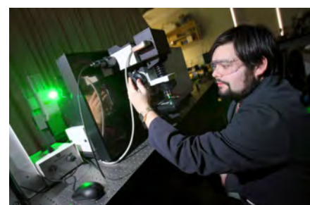
Tim Gonzalez demonstrates how the Raman microscope can be used for to study vibrational, rotational, and other low-frequency modes in a system to identify chemical bonds
