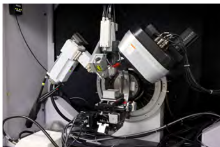
The X-Ray diffractometer (XRD) performs non-destructive analytical techniques which reveal information about the crystallographic structure, chemical composition, and physical properties of materials
