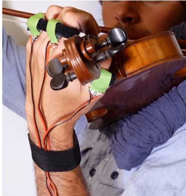
Figure 1. Vibrating rings worn by the violinists during the experiment.
