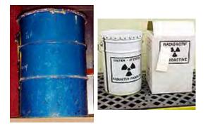
The waste containers that are collected from the radioisotope laboratories are transferred to the McGill Waste Management center periodically as Industrial Packages, Type IP-1 (transported under excusive use). The wastes are classified UN 2912, Radioactive Material, Low Specific Activity (LSA-I), non-fissile or fissile excepted.
