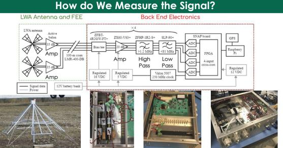
An antenna is used to measure galactic foregrounds. The signal is passed through electronics that amplifies and filters it. Our SNAP board changes this to a digital signal and is stored in hard drives using a Raspberry Pi.
